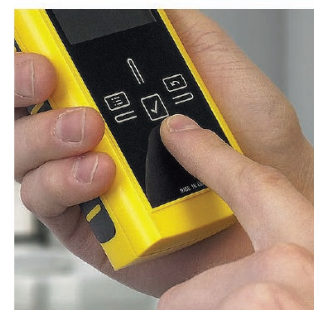
T610 and T660 come with a continuous surface made of highly scratch-resistant Blanview special glass and capacitive touchscreen control panel.
